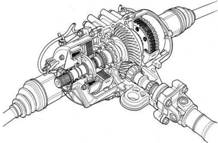
A connection from the ring gear to each wheel's half-shaft is made by left- and right-side clutches. Each drive clutch consists of three elements: an electromagnetic coil, a ball-cam device, and a set of 19 wet clutch plates which are similar in design to clutches used in an automatic transmission. Ten of the plates are splined (mechanically connected) to the ring gear while nine of the plates are splined to a half shaft. Left and right clutches are identical.
