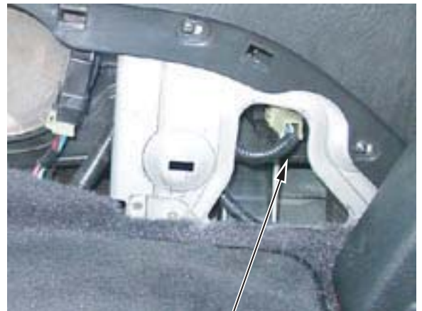
REAR POWER TRANSISTOR WIRE HARNESS CONNECTOR
