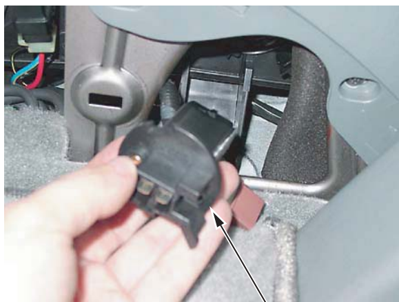
REAR POWER TRANSISTOR
