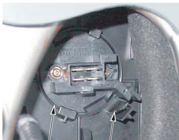
REAR POWER TRANSISTOR
